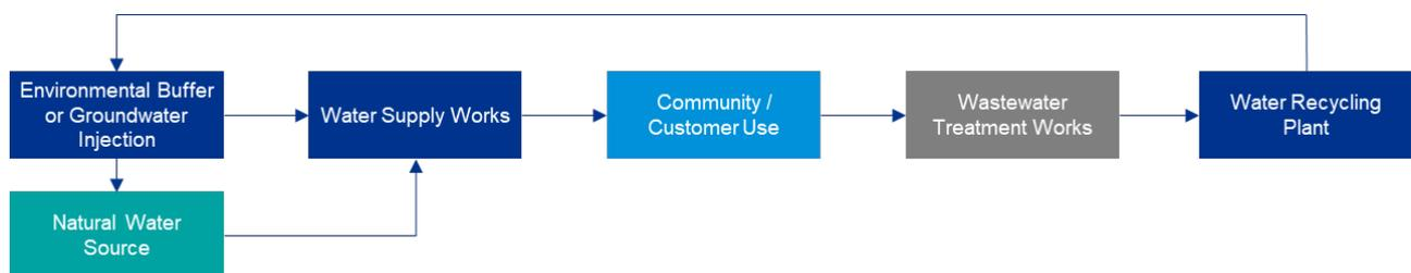
Figure 3 - Indirect water recycling process
