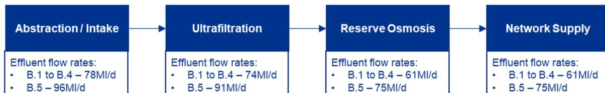
Figure 4 - Water recycling plant treatment process including effluent flow rates
