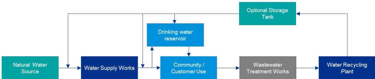
Figure 2 - Direct water recycling process
